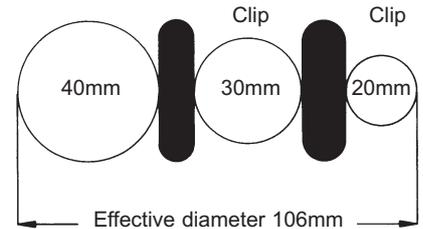
Add 6 mm for every small clip or 8 mm for every medium clip or 10 mm for every large clip. In each case the total diameter must not exceed the max. joint diameter of the kit. Use kit XAGA 550 122/30-xxx.
