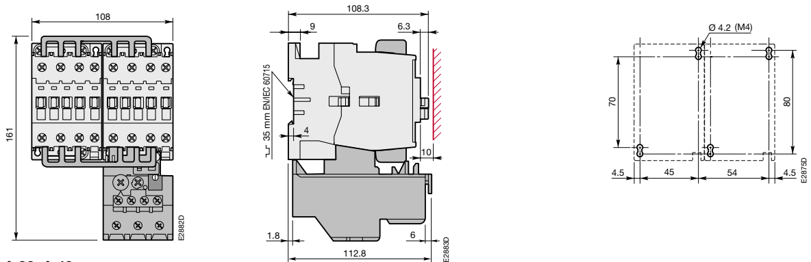
A 30, A 40 + BER 40 connection set + TA 42 DU thermal O/L relay
